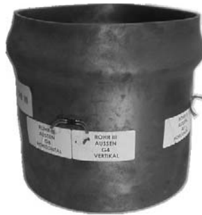
Fig. 10. Axially loaded pipe with L/D=1 after testing.
